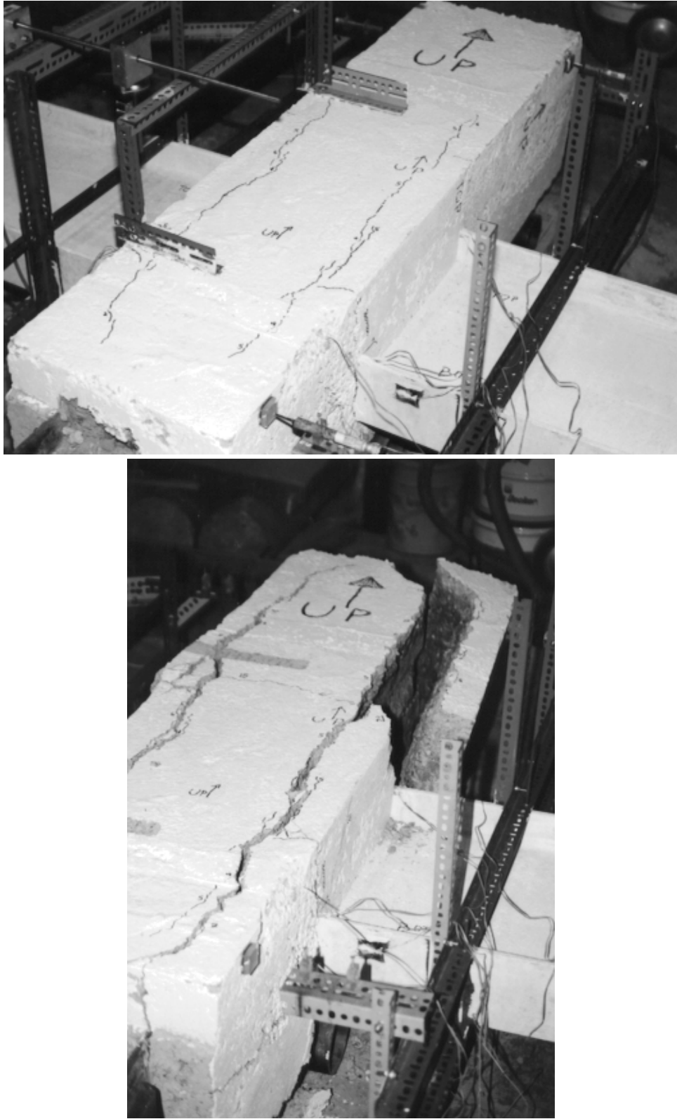
Figure 3. Behavior of non-retrofitted specimen with concrete encasement: (top) Visible cracking at early stages of testing; (bottom) Spalling of column fire-proofing near end of test.
